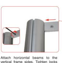
Attach horizontal beams to the vertical frame sides. Tighten locks using a 5mm allen key. If using rigid infill graphics, slide these in to position before tightening beams.
