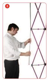
Attach the magnetic bars to the pop-up frame nodes
