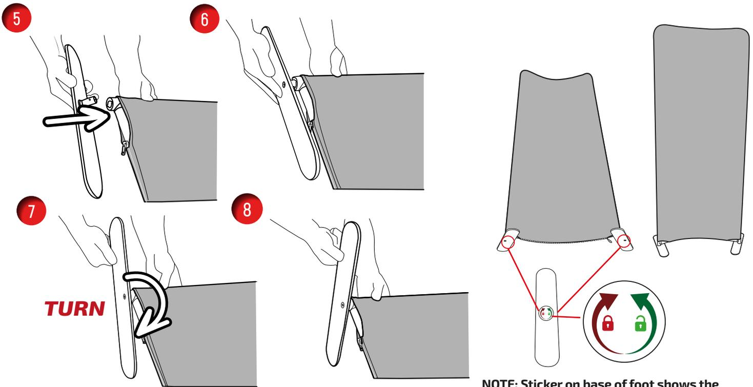
**NOTE:** Sticker on base of foot shows the directions for locking/unlocking foot
