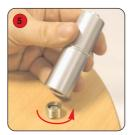
Fasten each standoff to the brass fasteners mounted to the top.
