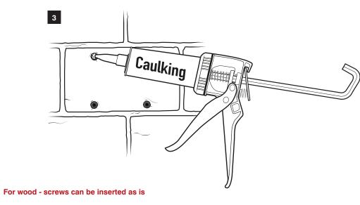
For brick - place a bit of caulking and wall plugs into holes before inserting screws
